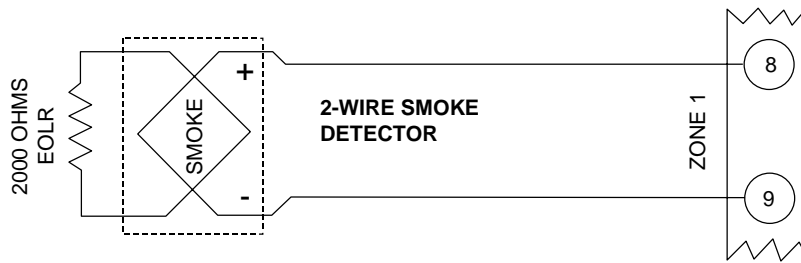
Figure 8. 2-Wire Smoke Detector Connected to Zone 1
